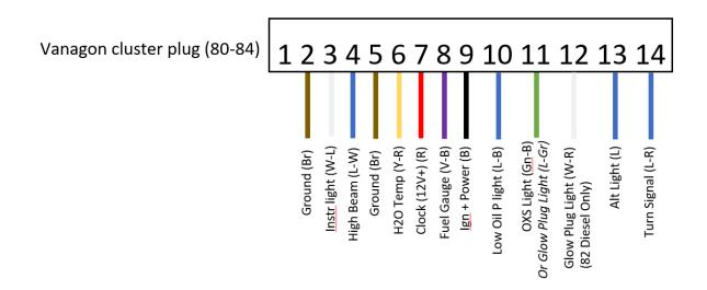
Move pins as necessary. Note: it may be necessary to cut wires and splice to repurpose unused pins.
